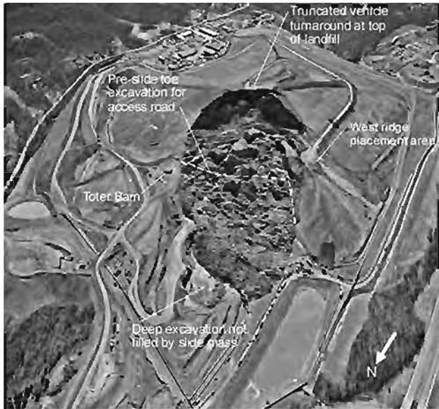
Figure 3. Sample problem – Aerial view of Cincinnati landfill failure (from Eid et al. 2000). (Reproduced by permission of the publisher, ASCE).
